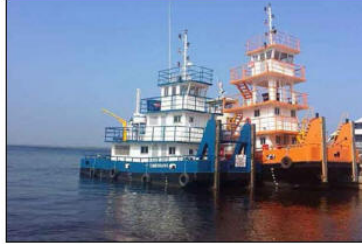
Figure 99 River pusher (WorleyParsons and PdB, 2022, /59/)
