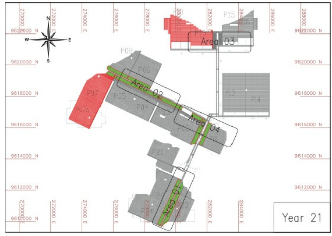
Figure 56 Start of mains on retreat with ramp-down of panel productions
