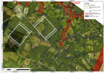
Figure 129 Illustrative layout of the brine Injection well locations (yellow points)
